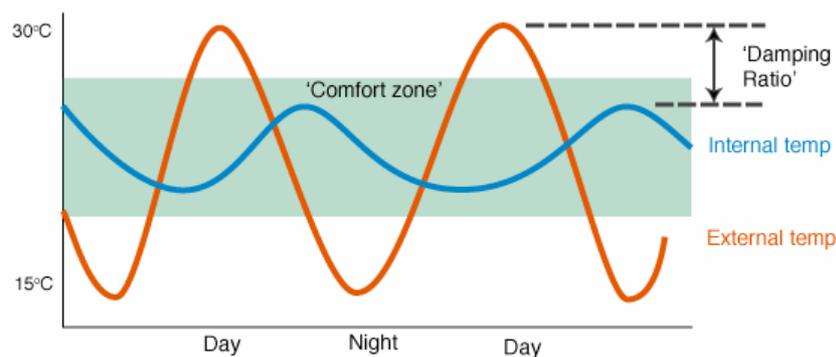
Figure 1: Temperature variations experienced by a construction
